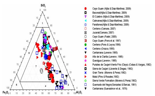
Figure 1. SiO<sub>2</sub>-Al<sub>2</sub>O<sub>3</sub>-Fe<sub>2</sub>O<sub>3</sub> plot for the non-nickeliferous weathering crust in Eastern Cuba. 1- silicic; 2- sialitic; 3- allitic; 4- ferrallitic; 5- ferric; 6- ferrisilicic; 7- ferrosialitic.
