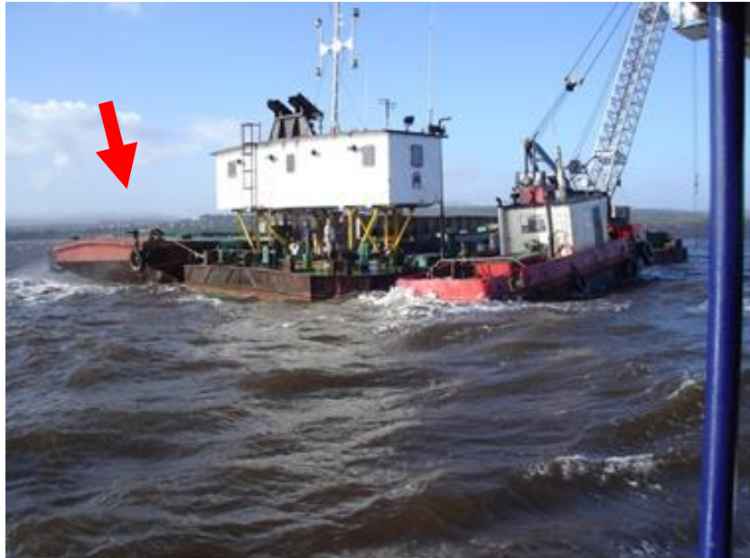
Figure 3. Barge for transporting and depositing the mineral, coupled to the extraction platform.
