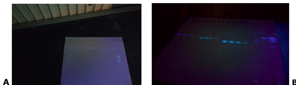
Figure 1. Chromatographic plates: sprayed with H 2 SO 4 (1:3) (a), illustration of the fluorescence of the standards (B2, G1 and G2) and of the contaminated samples (b).
