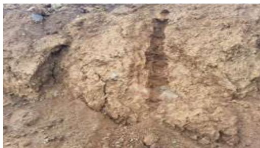
Figure 4. Groove-method sampling of the lateritic ore in the stockpiles of the platforms.
