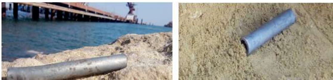
Figure 3. Sample a) exposed on the surface. b) when buried.
