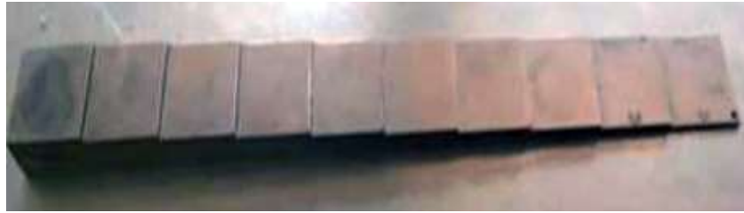
Figure 3. Step wedge from 1 to 10 mm with 1 mm steps.
