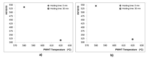
Figure 3. Variation of hardness for HAZ in double cycle. a) (1350 + 1000) °C/5; b) (1350 + 1000) °C/12 s.
