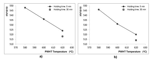
Figure 2. Variation of hardness for HAZ in simple cycle. a) 1000 °C/12 s; b) 1350 °C/12 s
