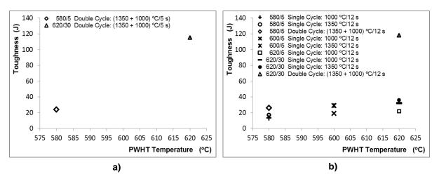
Figure 5. Variation of toughness of HAZ for: a) Double cycle and 5 s of cooling time; b) Single and double cycles and 12 s of cooling time
