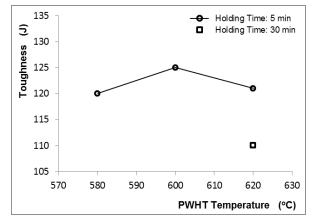
Figure 4. Variation of toughness for BM after different PWHT and holding times
