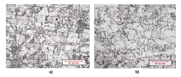
Figure 6. Typical microstructure for BM. a) In as-received condition, b) Postweld heat treated at 620 °C. Magnification: 200 x
