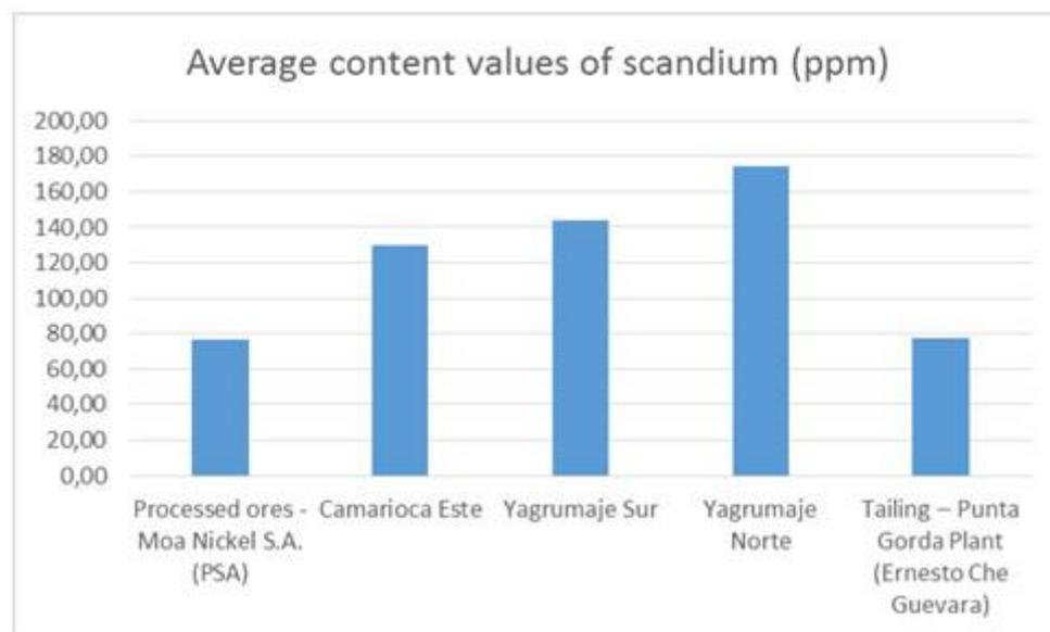
Figure 5. Values content of scandium (ppm) reported in the lateritic nickel and cobalt ores from Moa mineral district and in the tailing of Ernesto Che Guevara nickel plant. Source: Data from the Ministry of Energy and Mines (2015) and the Institute of Geology and Paleontology-Geological Survey of Cuba (2016). Modified by the authors.
