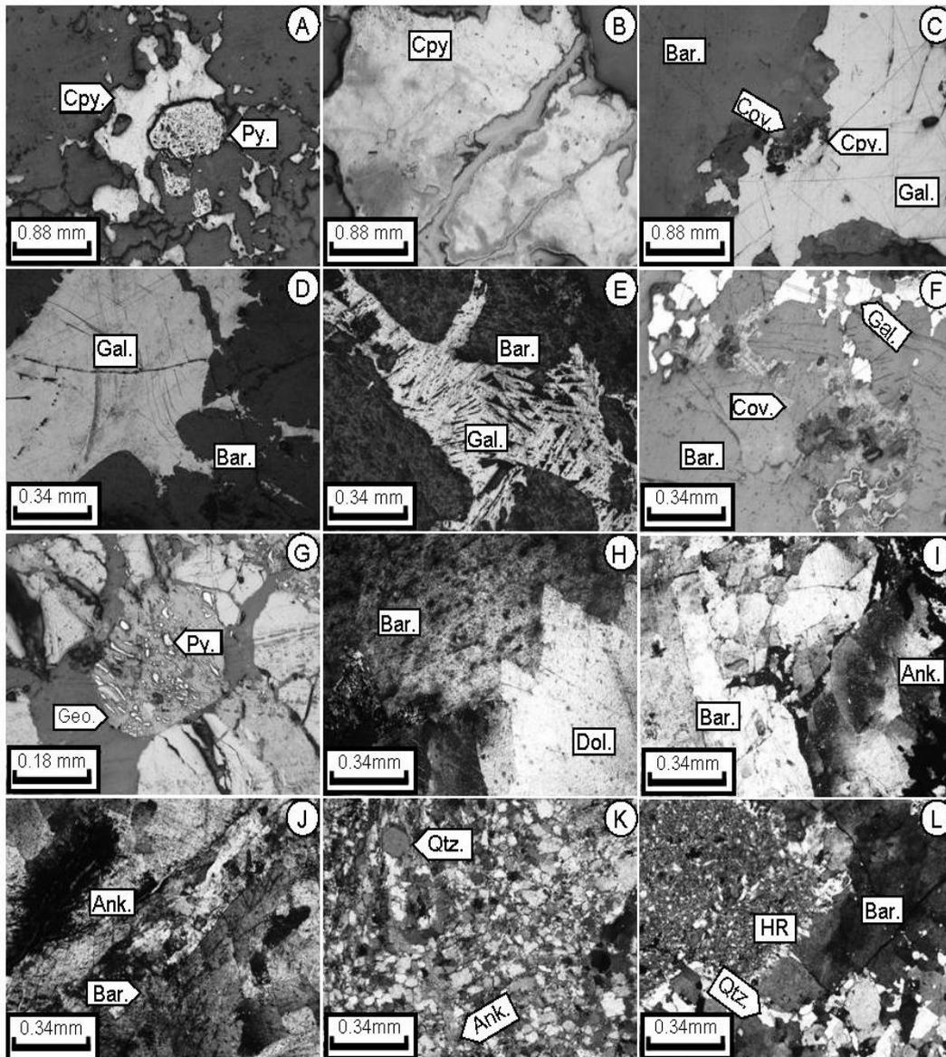
Figure 4. Photomicrographs of metallic and non-metallic minerals: (A) Pyrite in contact with chalcopyrite; (B) Tarnished chalcopyrite; (C) replacement of chalcopyrite to galena; (D) Galena without pit; (E) Elongated bayonet-shaped pits in galena; (F) Covellite around a galena; (G) Pyrite islands in the goethite matrix; (H) Coarse-grained euhedral dolomites; (I) undulatory extinction in ankerite; (J) Barite veinlet in ankerite; (K) Pre-ore forming quartz aggregates; (L) Secondary quartz
