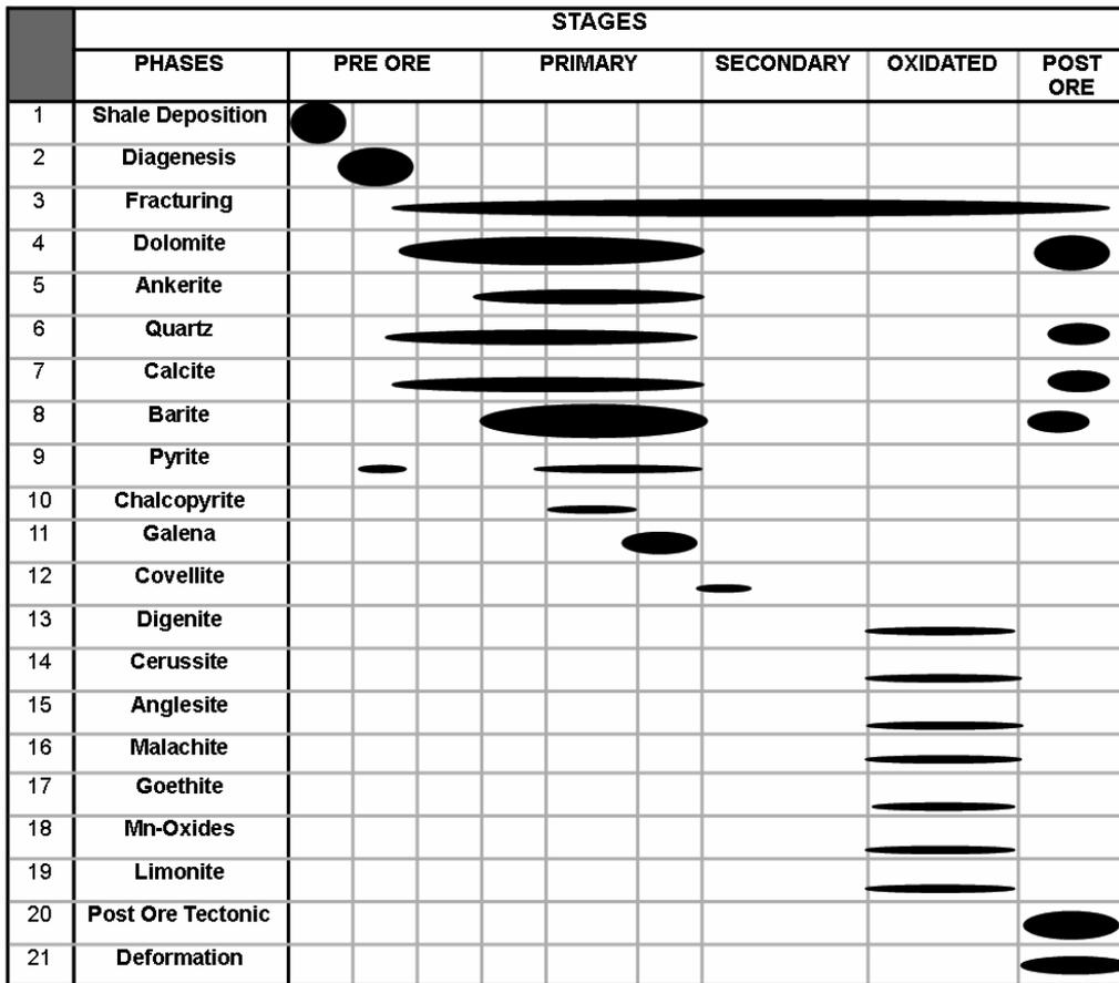
Figure 5. The arrangement of the mineralization and dependent events
