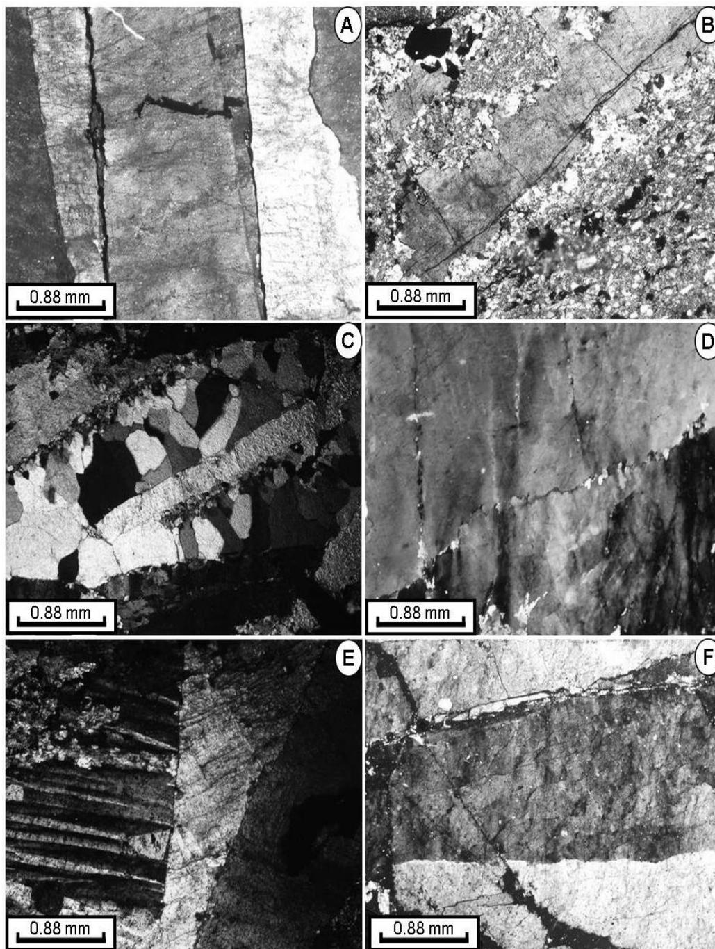
Figure 3. Photomicrographs of barites: (A) euhedral - subhedral coarse grained barites; (B) epigenetic relation with regard to mineralization host rock and barite; (C) geode aggregates of barite; (D) Concrete relation between barite crystals; (E) undulatory extinction and poly-synthetic twinning - poly lamellar bounding in barites; (F) tabular barites.
