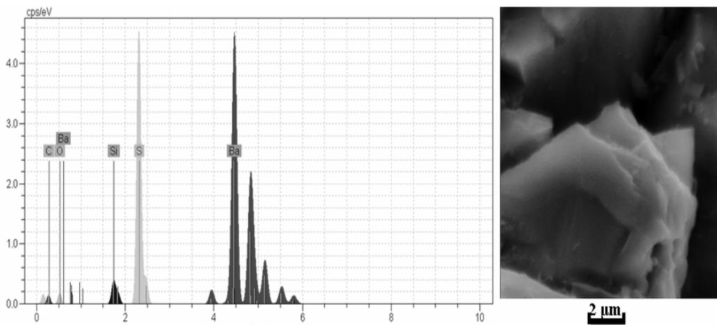
Figure 6. SEM image of tabular barites and its EDS spectrum.
