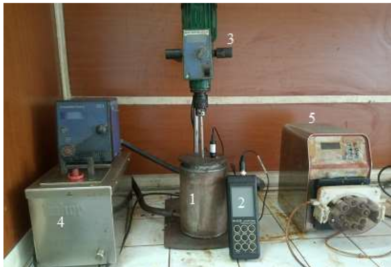
Figure 2. Experimental setup for atmospheric pressure leaching with sulfuric acid.
