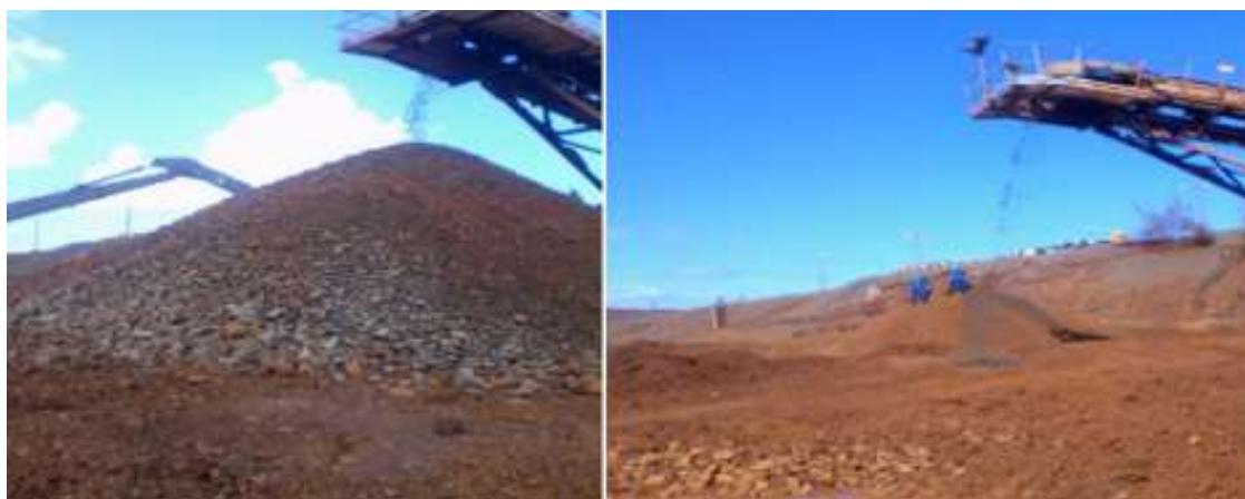
Figure 1. Serpentine reject deposit at the pulp preparation plant of the HPAL nickel company.
